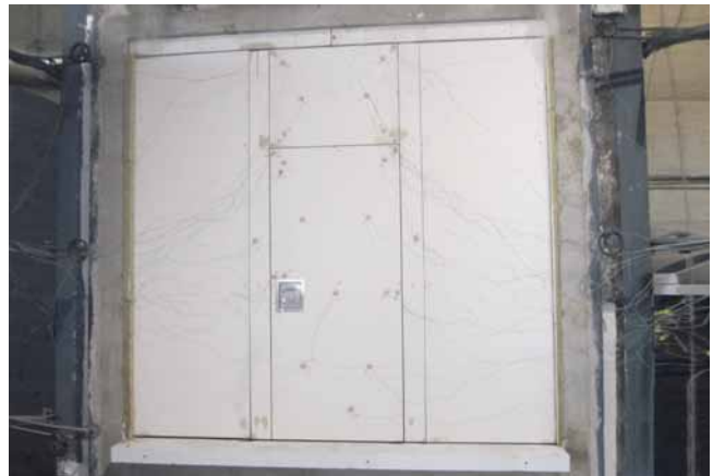
To determine the fire protection class, one wall face of the Variflex EI 30 with integrated pass door was exposed in a test laboratory to the direct flame of a test fire for half an hour.
